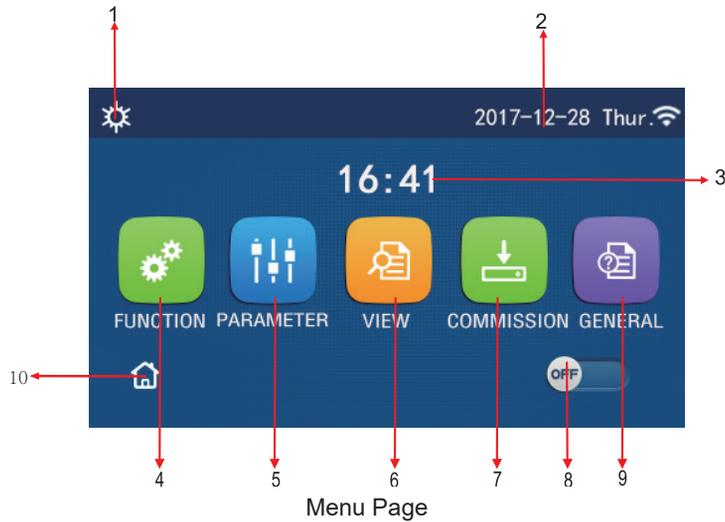
Above the menu, the corresponding icon will be displayed based on the mode and status of the controller.
