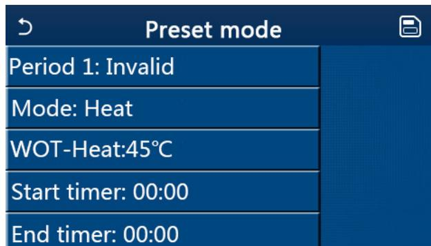
The option “**Mode**” is used to preset the mode; “**WOT-Heat**” is used to set the leaving cold/hot water temperature; “**Start timer**”/“**End timer**” is used to for time setting. After that, by touching the “**Save**” icon, all settings will be saved.
