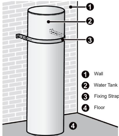
The minimum clearance from the water tank to combustible surface must be 500mm.
