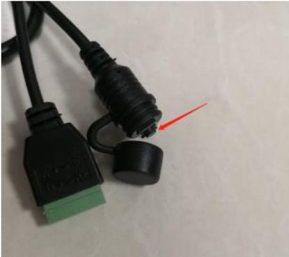
Click the button, the green light of the module flashes quickly, and it enters the distribution network mode.
